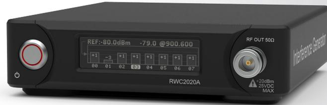
RWC2020A is an interference generator being able to be used for the purpose of various tests or measurements, e.g. the Listen Before Talk (LBT) test, the Gateway Non-regression tests, the Intermodulation Immunity test and so on. It can generate up to eight multi-tone signals with different output levels per each tone for the LBT test and two tones of up to 20MHz distant for the Intermodulation Immunity test.
